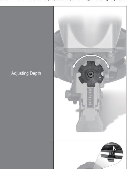
The depth that the fastener is driven can be adjusted using the depth adjustment wheel on the nose of the tool. The depth of drive is factory adjusted to a nominal setting. Test fire a fastener and check depth. If a change is desired:
