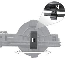
1. Loosen the adjusting screw (N) and slide the guide (H) to desired position.
