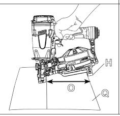
The guide (H) can be used as an aid to position the shingle being nailed a specific distance (O) from the front edge of the previous row of shingles (Q) as shown.
